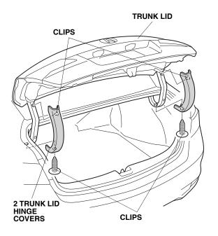
3. Remove the three clips from each trunk side liner.
