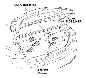
4. While wearing eye protection, use a 9mm drill to enlarge the two upper clip holes. Wrap tape around the drill bit 15 to 20 mm (0.6 to 0.8 in.) from the tip of the bit.
